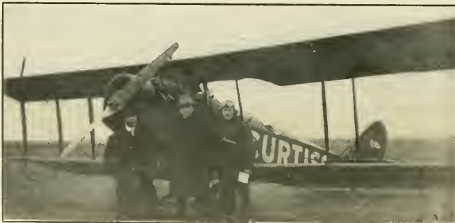
© U. S. Army Air Service Fig. 1—Reed dinalumin propeller D-4 mounted on Curtiss JN with OX5 engine
